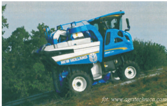
Rys. 9. Samojezdny kombajn do zbioru winogron V6060 Fig 9. Self-propelled grape harvester V 6060 - harvesting grape with the maximum safety
