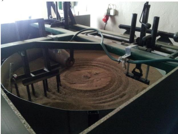
Fig. 2. The „rotating bowl” unit: a) scheme [5]: 1 - transmission, 2 - engine, 3 - running rail, 4 - bowl, 5 - holder of the sample, 6 - supporting frame, 7 - roller: 8 - frame of the bowl, 9 - main frame, b) view [6]
