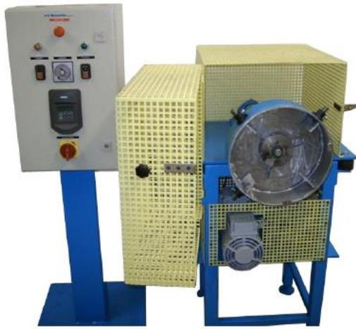
Fig. 1. CIAT machine for continuous abrasive testing [3]
