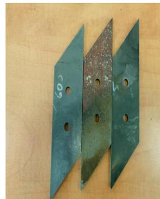
Fig. 3. Sample tested in the abrasive test [7]; a) scheme, b) view
