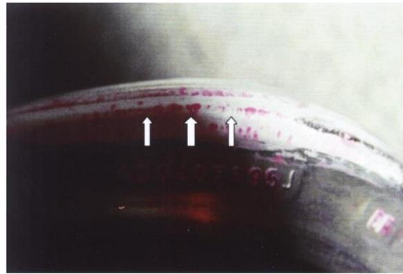
Fig. 9. So called striped cracks in deformed suspension arm detected by penetrant method [7]
