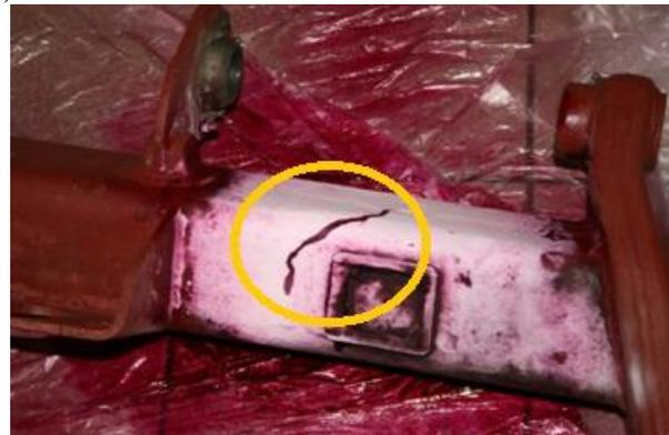
Fig. 6. View of BPW axle of semi-trailer with suspicion of cracks (a) and detected crack by penetrant method (b) [7]
