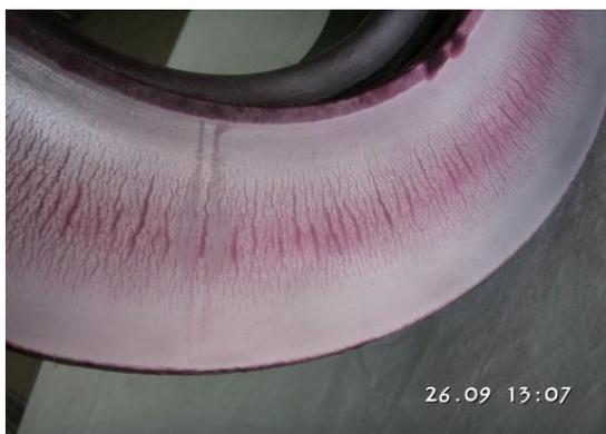
Fig. 8. A fragment of the brake disk tested by coloured penetrant technique [7]
