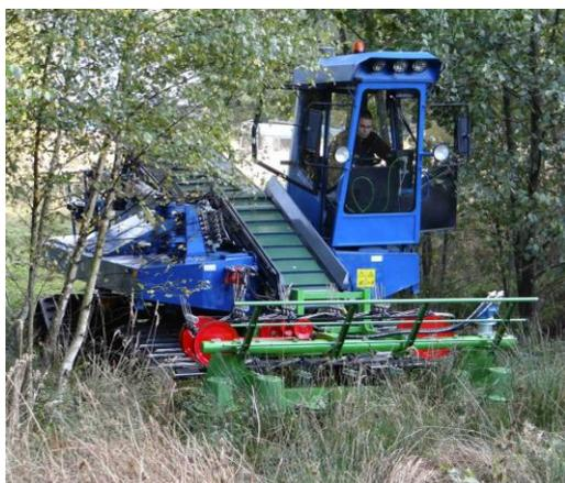
Fig. 1. The tracked vehicle during sedge cutting trials - PIMR-BE archives
