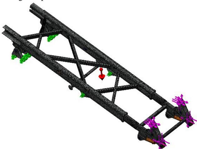
Fig. 11. The loading transporter unit model, initial conditions prior to strength analysis - PIMR-BE archives
