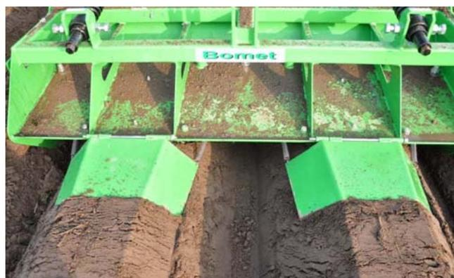
Fig. 5. Cover plates forming ridges [3]
