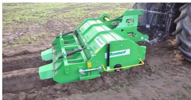
Fig. 1. Aggregate suitable for ridging potatoes during work [3]
